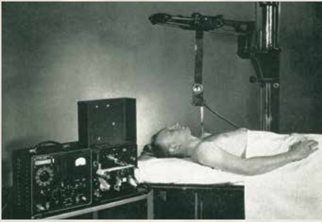
Apparatus designed by Rosalyn Yalow to measure thyroid uptake of radioactive iodine.
